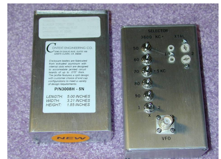
Figure 6. Crystal and VFO interface box to be plugged into existing crystal sockets
