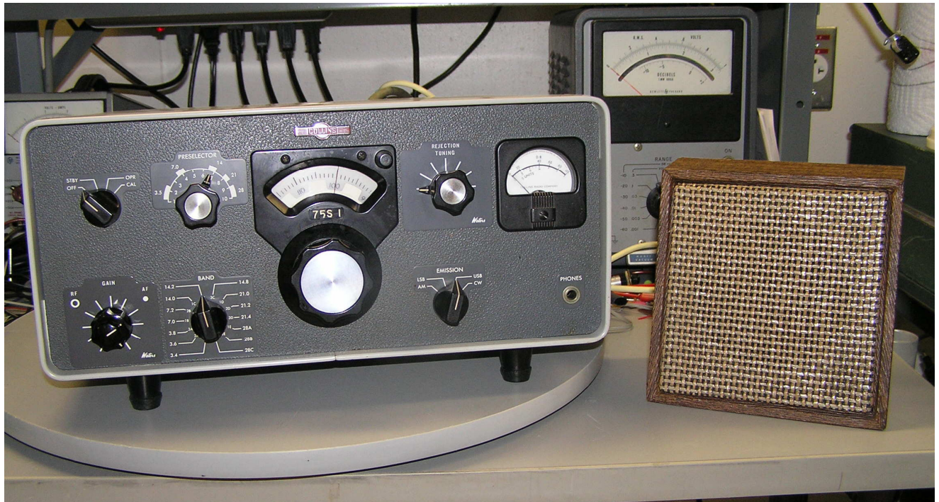
Figure 1. Typical 75S-1 receiver set up on the test bench with test speaker and easy access turnstile.
